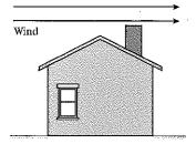
Air Flows in the window and out the chimney. The high speed of the air at the chimney results in a lower relative pressure.
