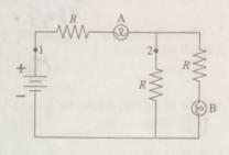
b. Bulb A is replaced. Bulb B is then removed from its socket. What happens to bulb A? Does it get brighter, stay the same, get dimmer, or go out? Explain.
