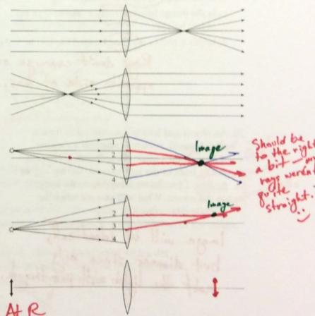
18. An object is near a lens whose focal points are marked with dots.
