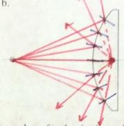
22. An object is placed near a spherical mirror whose focal point is marked.
