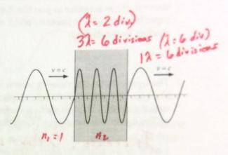
2. A light wave travels from vacuum, through a transparent material whose index of refraction is n = 2.0, and back to vacuum. Finish drawing the snapshot graph of the light wave at this instant.
